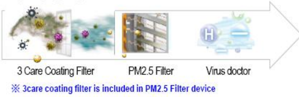
Air purifying stage of PM2.5 model
