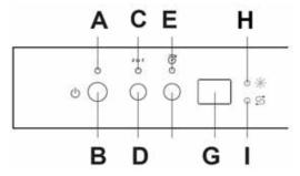
You can check the malfunction, when the time-remaining indicator "G" displays one of the signs as following.
