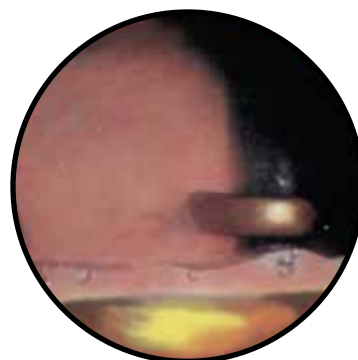
FIGURE 6-7: Normal run with heat. Oil level is maintained thereby assuring effective lubrication for compressor bearings.
